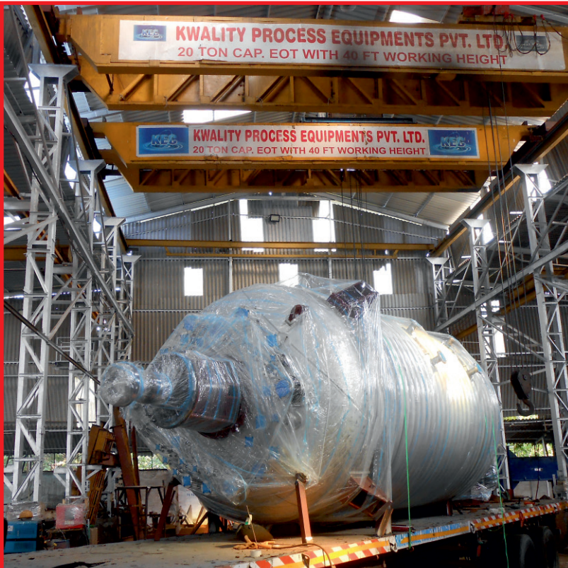
30 KL Limpeted Reactor
