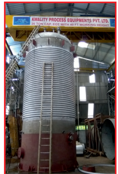
62 KL Limpeted Storage Tank
