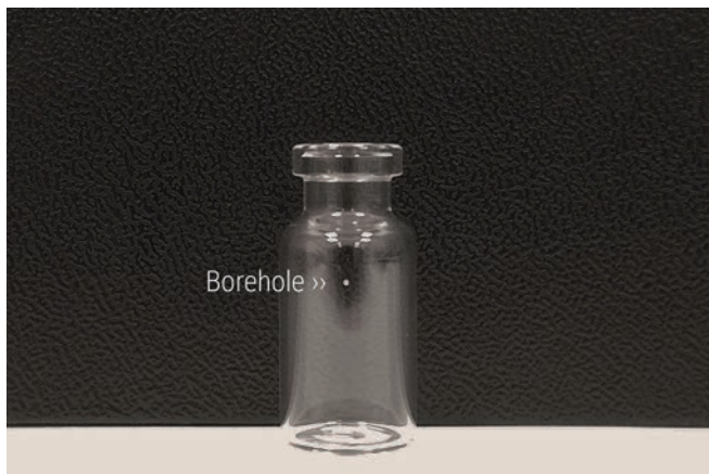
Leakage drilling in glass
