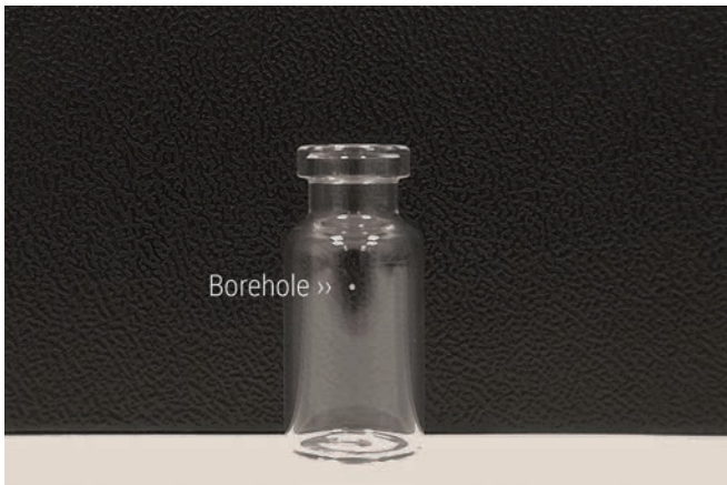
Leakage drilling in glas
