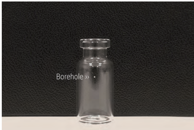
Leakage drilling in glass
