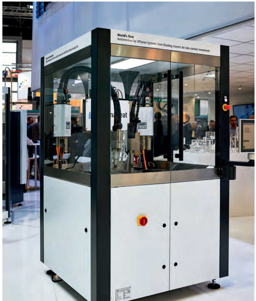
The new plasma treatment unit is highly compact as it no longer requires a 6-axis robot or additional linear axes. Picture: © Plasmamatreat, Jan Dufelsiek
