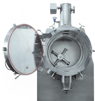
Planex® System: multi-patented paddle vacuum dryer with ZeroFriction® planetary movement eccentric agitator
