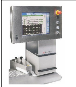
Among others, POLYPHEM wt inspects colour, form, size and positioning of tablets, capsules and dragees in blister packaging
