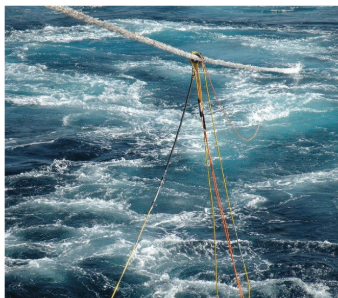
Figure 5: PAM towed array entanglement with lead-in
