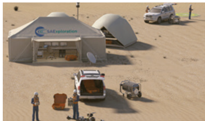
The automated seismic acquisition system uses autonomous drones and a ground vehicle to drop off and retrieve seismic sensors without human intervention.
