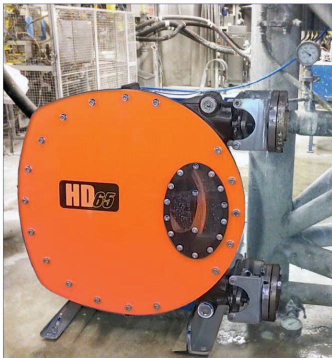
Peristaltic (hose) pumps are able to operate safely, efficiently and reliably in many of the harsh liquid-transfer applications that are prevalent in oil-and-gas production.
