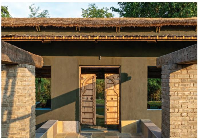
By virtue of its proximity to the Chandrapur Super Thermal Power Station, the by-product fly-ash is normally a nuisance; the resort's response to this - fly ash bricks were incorporated into the architecture of the resort.
