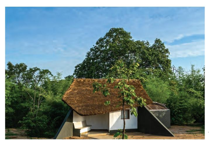
All built form has been planned around the existing vegetation on site. The grass thatched roofs, experiments with mud plastered walls and the interplay of color through natural stone have been emulated from the local Gondi architecture.
