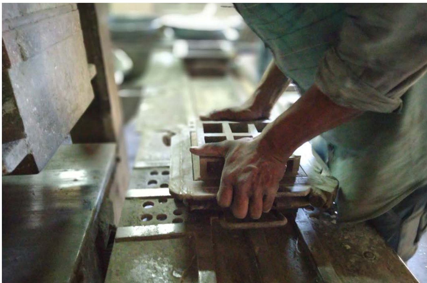
The Carbon Tile is made using a hydraulic press to fuse together carbon, cement and natural materials.
