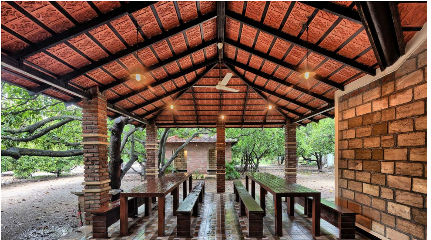
Local 'thin' brick columns and terracotta tiled roofs create a semi-open dining area.
