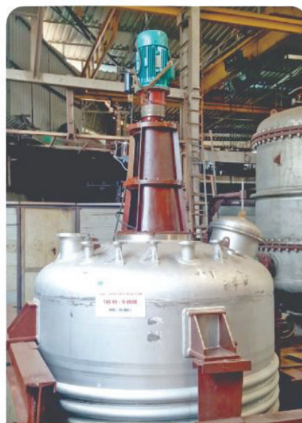
25 KL SS 904L Reactor
