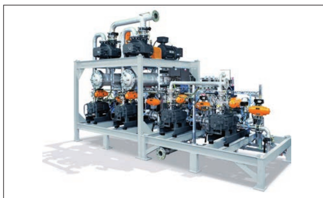
Figure 4: Custom-engineered vacuum system with PANDA and PUMA vacuum boosters as the first stage and COBRA screw vacuum pumps as backing pumps Source: Busch Group.
