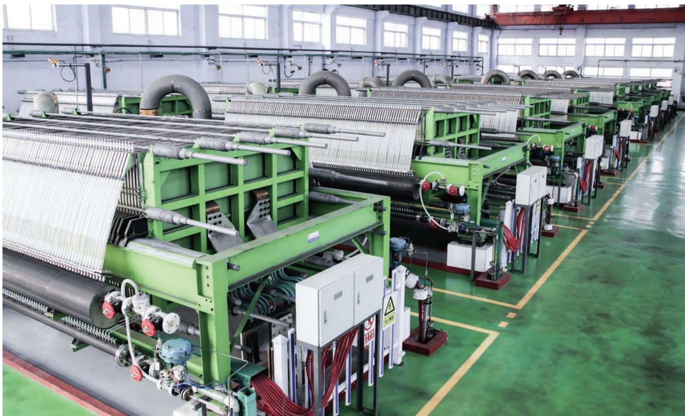
Bipolar ion exchange membrane process electrolyzer
