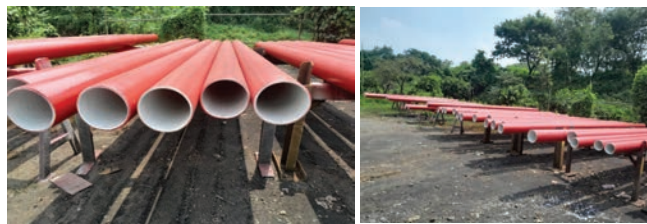
Internally and externally coated pipes with Glass Flake Epoxy.
