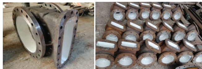
Glass flake epoxy coated valves.
