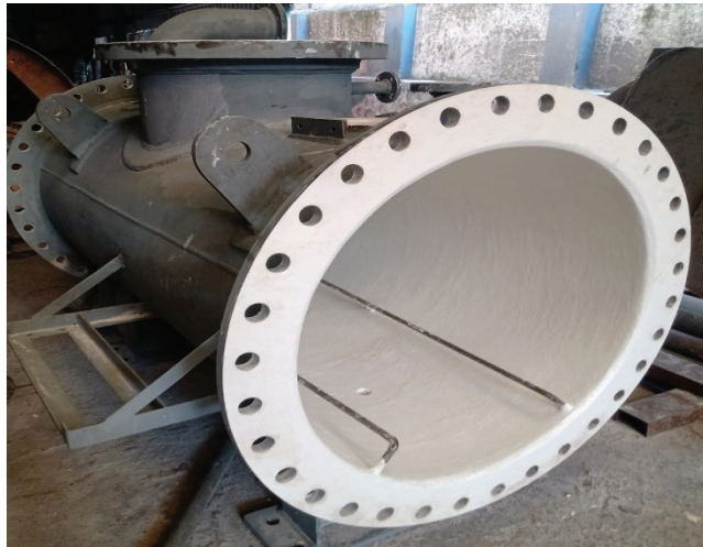
MS tanks lined with FRP for the anodizing and powder coating industry.
