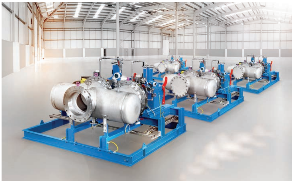
LEWA pulsators for the chemical and pharmaceutical industries
