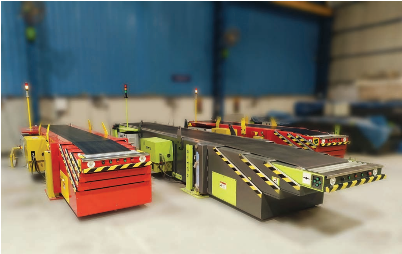
Telescopic conveyor from Atmos Systems
