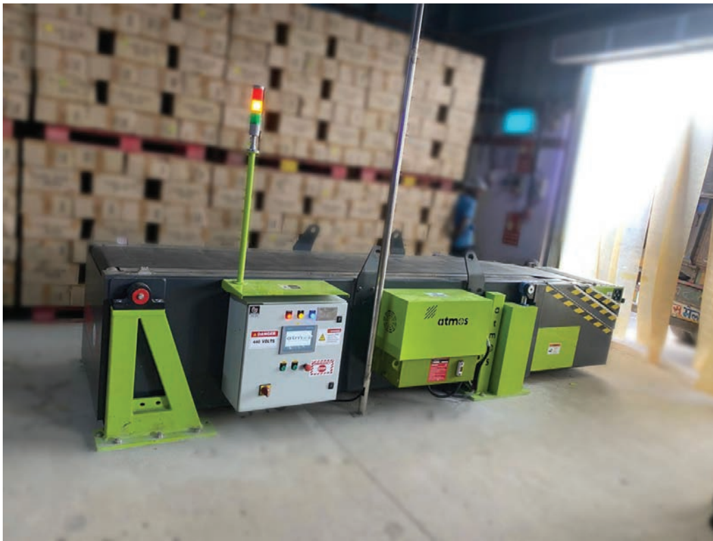
Telescopic conveyor from Atmos Systems
