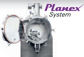
Horizontal paddle dryer with eccentric agitator
