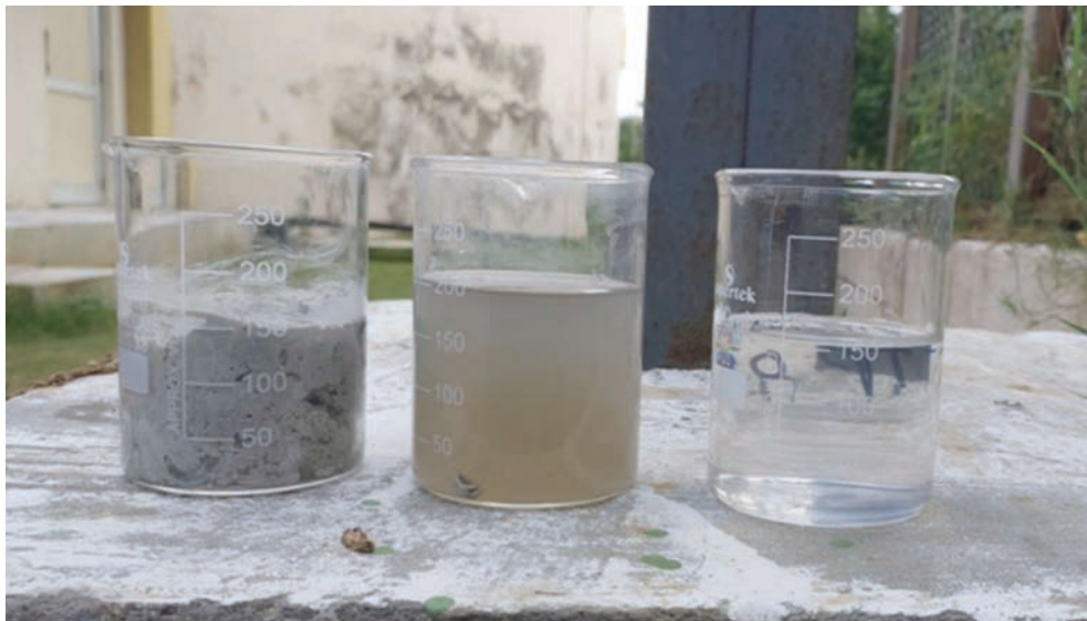
Sample of fat sludge (Left), digester outlet water (Centre) and final treated water outlet (Right)
