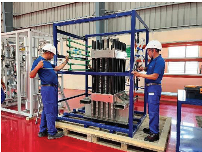
1MW PEM Electrolyser being assembled at GreenH factory, Jhajjar, Haryana
