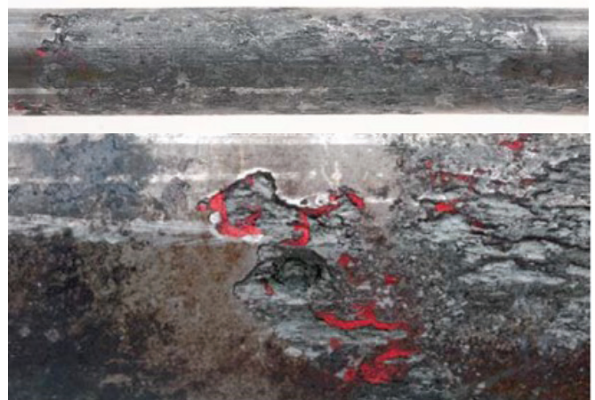
Underdeposit corrosion of tubes – sulfur found in deposits.
