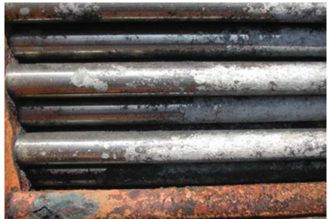
Duplex steel has a good surface in comparison with corroded carbon steel tie-rod (red colour tube at bottom) in overhead condenser after seven years of service.
