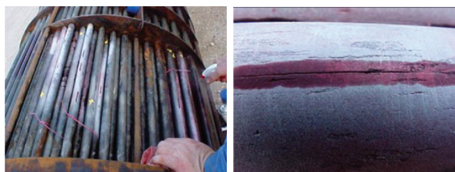
Stress corrosion cracking in Cl and S.
