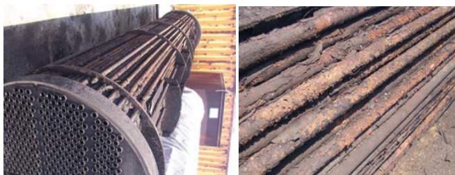
Carbon steel tube bundle after three years in service in overhead condenser, waiting for retubing.
