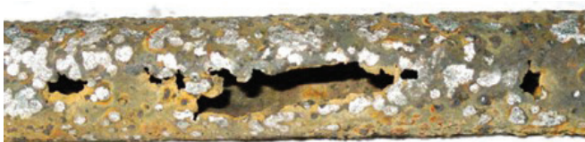
Failure due to general corrosion and formation of sulfides.
