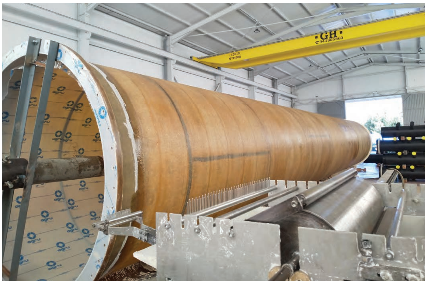
ECTFE dual-laminate part of the stack during the lamination process
