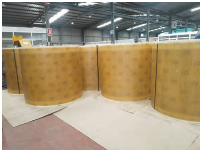
ECTFE sheets including a conductive element in the welding area
