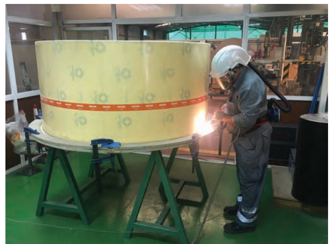
Hot-gas welding of ECTFE fabric backed sheets
