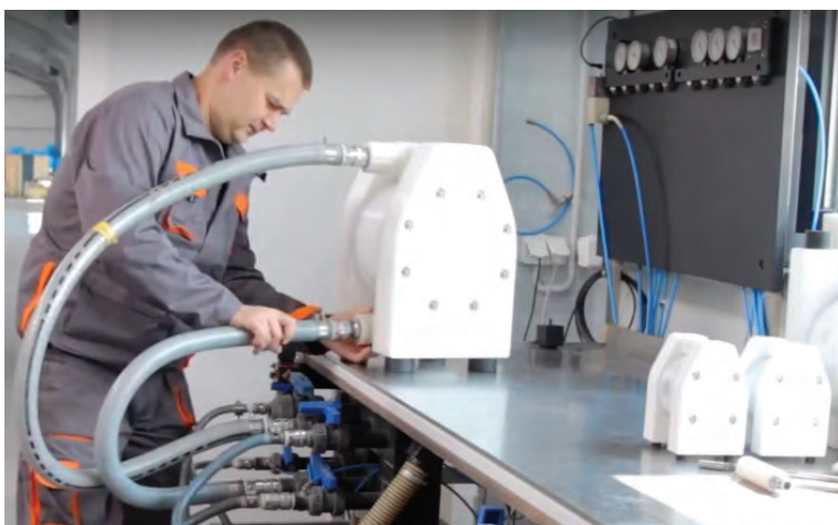
Fig 1: Dellmeco employee conducting Hydro Test of Pump
