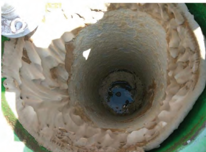
Removed Scale collected in the reactor
