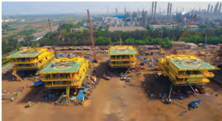
Production Deck Modules ready for dispatch from the company's Modular Fabrication Facility in Hazira, India
