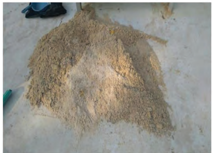
Loose scale easily scrapped off from reactor
