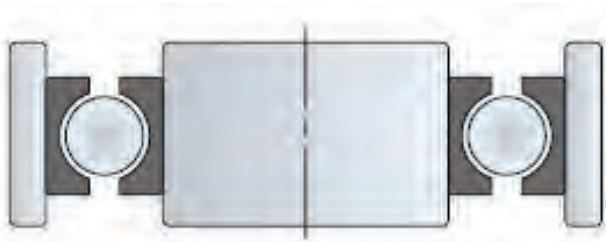
Pic. 2: Bearing without a preload : Clearance between components can cause vibration & wear
