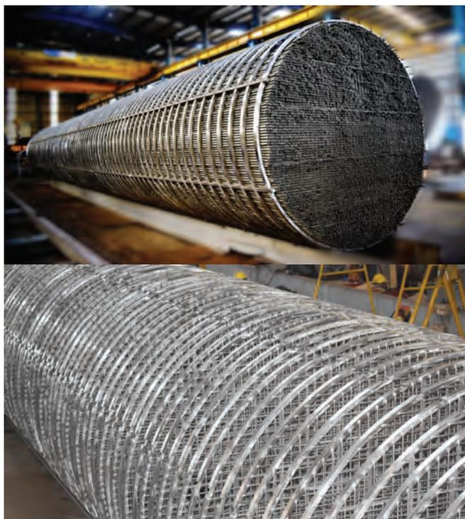
Fig. 3: Tube & Rod Assembly
