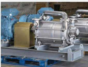
**Two-stage Liquid ring vacuum pump**
