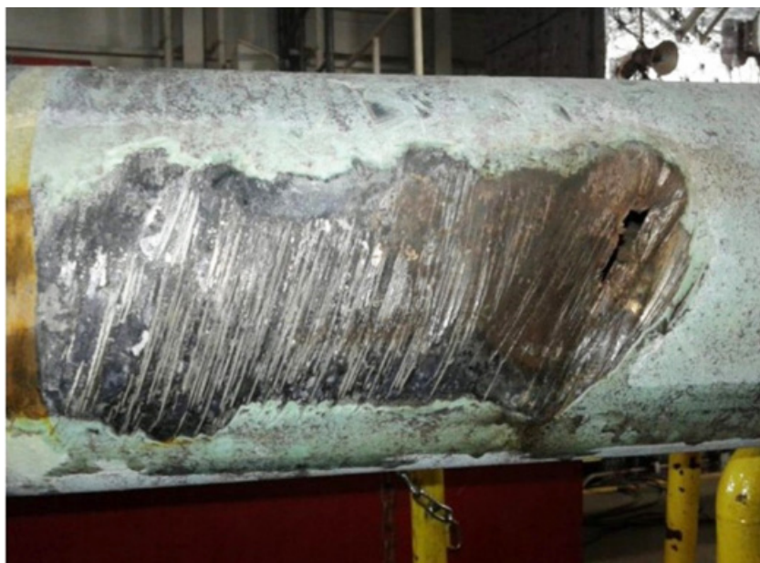
Figure-2: Physical appearance of the anomaly on verification
